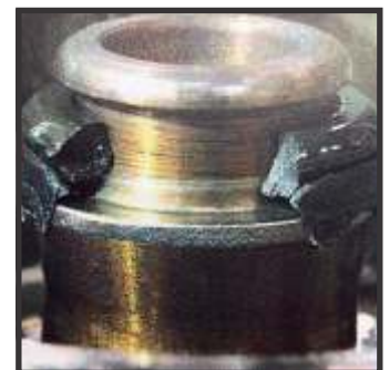
Bad Oil Rail Seal
