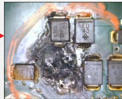
This main board has burnt components and a significantly damaged printed circuit board.
