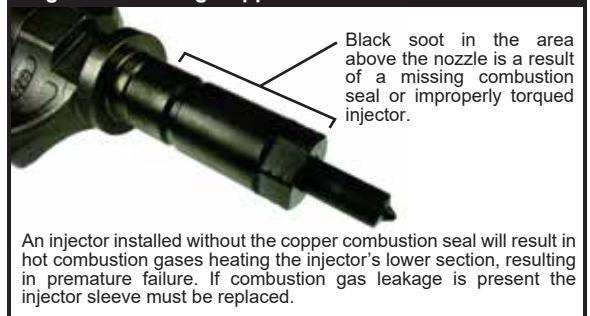
Figure 4 - Missing Copper Combustion Seal
